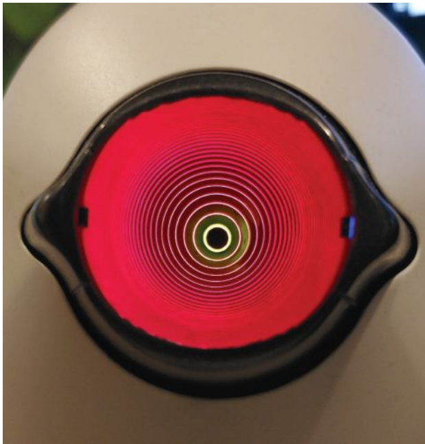
Placido disc corneal topography seen from a patient's bird eye view. Placido disc evaluation is valuable in assessing the corneal contour and the quality of ocular surface. It can guide the selection of specialty CL design.
