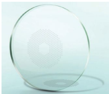
The Miyosmart lens from Hoya (left) contains a 9.4mm diameter central zone of distance vision surrounded by a honeycomb-like pattern of 396 defocusing lenslets of +3.50D power, equally distributed. Essilor's Stellest (right) is designed with a similar 9mm central zone. However, the surrounding is made of highly aspherical lenses, varying in distribution and power vs. distance refractive error correction, along 11 segmented rings, to generate a volume of defocus following the retinal shape.
